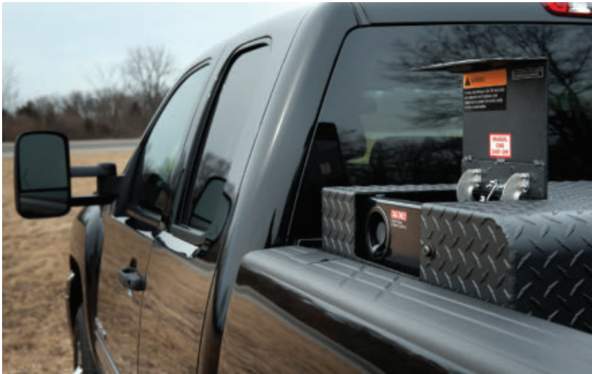
General Motors' CNG capable Chevrolet Silverado and GMC Sierra 2500 HD Extended Cab is equipped with the Vortec 6.0 L V8 engine. The trucks are built in Fort Wayne, Ind., then sent to IMPCO Automotive, Union City, Ind., for installation of the bi-fuel system.
